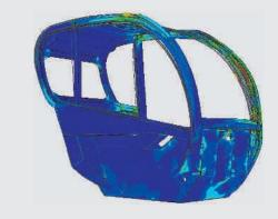
ROPS-FOPS approved cab designed with safety cell to prevent deformation in the event of vehicle overturn or a heavy load falling on the cab.
